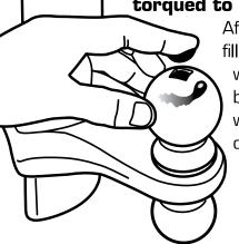
After installation, fill 1/2" drive sockets with a quality bearing grease, which can be dipped out and used to grease ball surface during towing.
